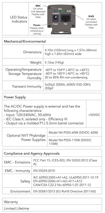
\*Important Note: Distance will often be shorter due to power supply capacity and wire voltage-drop. See Maximum Per-Camera Wire Distance Chart on Page 5. WARNING: For safety, never use more than two power supplies. Never exceed 120 watts.
